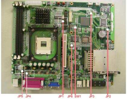
Figure 3.1: Jumpers on the IPPC-9151 motherboard
